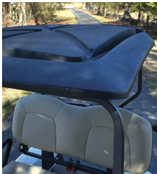
Injection molded roof with grab handles
